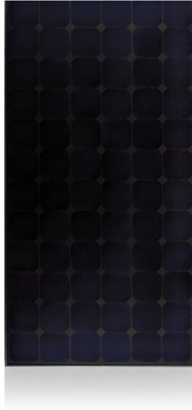
**The SunPower 220 Solar Panel provides a revolutionary combination of high efficiency and attractive, uniform appearance.** Utilizing 72 next generation SunPower all back-contact solar cells and an all-black backsheet, the SunPower 220 elegantly delivers an unprecedented total panel conversion efficiency of 17.7%. The panel's reduced voltage-temperature coefficient and exceptional low-light performance attributes provide outstanding energy delivery per peak power watt.
